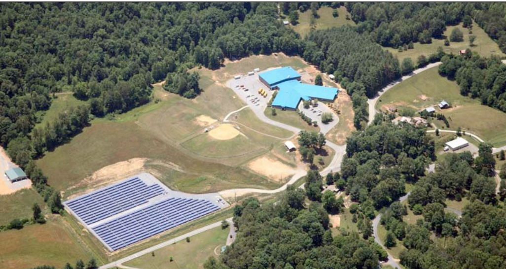
At the 999 kW Martins Creek installation, errant golf balls and a nearby bird sanctuary call for more regular cleaning and inspection.
